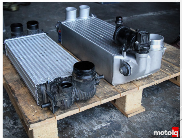
OEM intercooler (left) and the Garrett PowerMax intercooler (right). The Garrett intercooler is 83% larger than stock.
