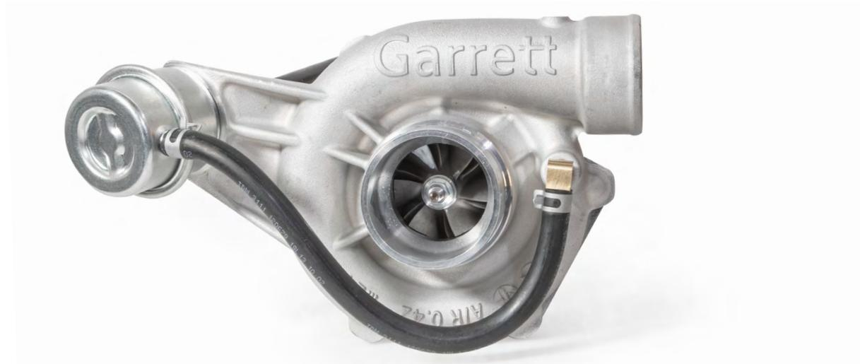
Garrett | Classic Turbo incorporates modern engineering with direct-fit installation for the iconic Lancia Delta HF Integrale 8V, 16V | Lancia Dedra | Alfa 155 2.0 Q4 | Fiat Coupe 16V. The modern journal bearing rotating group utilizes a 360-degree thrust bearing for improved reliability. Garrett integrated the actuator bracket into the compressor housing to strengthen the turbocharger. This turbocharger includes a gasket kit for a direct-fit installation.
